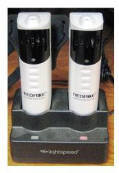
Check the power strip mounted inside of the lower back part of the media cabinet. Follow the cradle's power cable and make sure it is plugged into the power strip and also into the back of the cradle.
